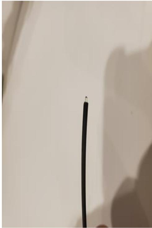
Step 8 Using a lighter flame finish the fiber on the stripped end of each of the 3 leads, hold the fiber near the side and base of the flame till you see the fiber start to ball up. The fiber only needs to be held close to flame, never contact the fiber to the flame and DONT over do it, the flame only needs to slightly
