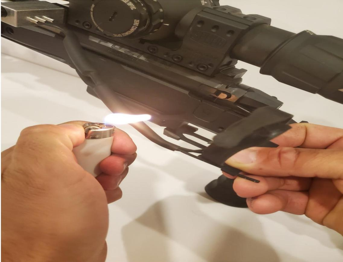
Step 12 Reinstall the leads on the gun and trim the leads about 1/16" past the ocular fiber rear housing, remove the fibers 1 more time from the rear housing, strip the outer housing back 1/8" and flame finish the ends same as you did in step 5. Reinstall the fibers into the rear housing making sure to insert them until the fiber is protruding past the back of the housing and you're done. (see pictures below)
