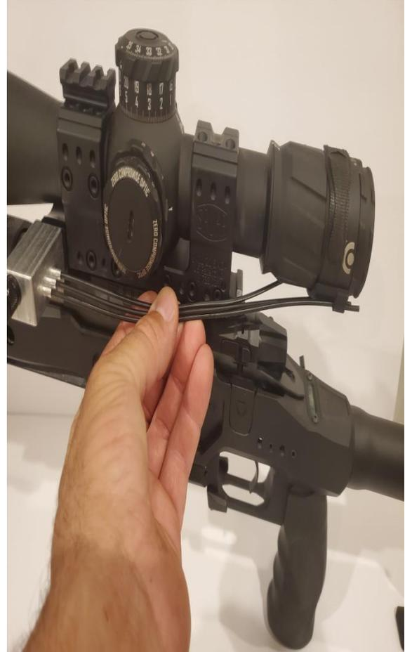
Step 10 determine the length of 1/2" heat shrink need to cover the main run of fiber bundle, measuring along the fiber bundle stopping and 5/8" short of either housing. Cut heat shrink to determined length, remove fibers from level housing and slide the heat shrink over the bundle then reinstall the ends into the housing and double checking you have reinstalled them in the appropriate locations.(see picture below)
